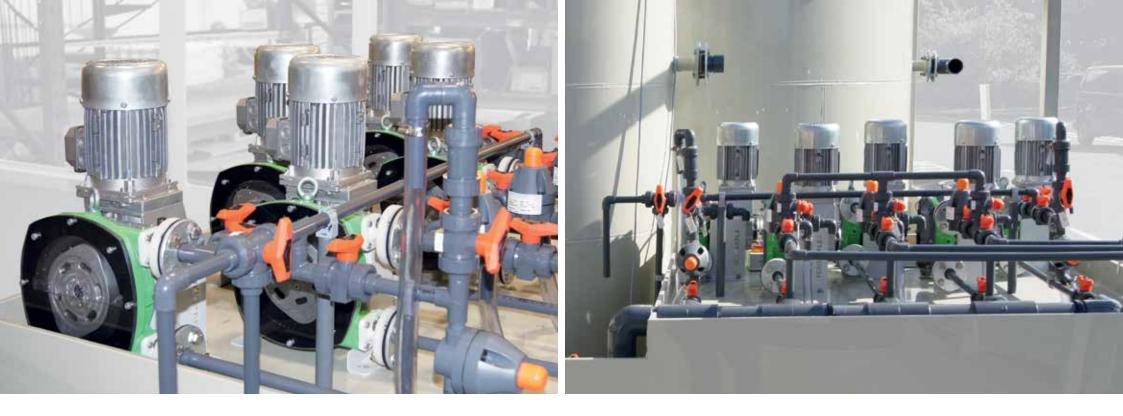
Peristaltic pumps are the ideal solution for many different applications. Due to their unique working principle these pumps can be used in the most diverse industries for a huge range of fluids and system conditions.
