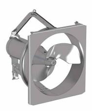
The B-MX is also suitable for circulation channels (slalom liquid manure channels). The submersible mixer sucks the liquid from the motor side and pushes it through the mixing tunnel thereby creating a circulation flow.
