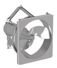
The B-MX is also suitable for circulation channels (slalom liquid manure channels). The submersible mixer sucks the liquid from the motor side and pushes it through the mixing tunnel thereby creating a circulation flow.
