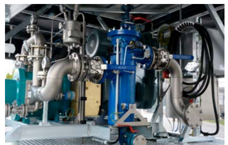
Filter system with differential pressure measurement
