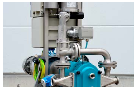
Overpressure protection by bypass with safety valve
