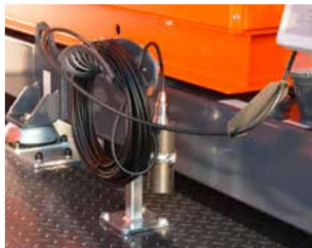
Automatic operation via level sensor
