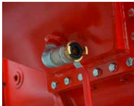
Drain for removal of residues
