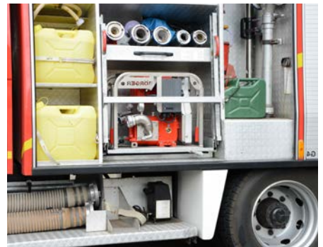
With a combustion motor, the pump can be carried by four persons
