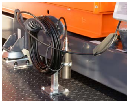
Automatic operation via level sensor
