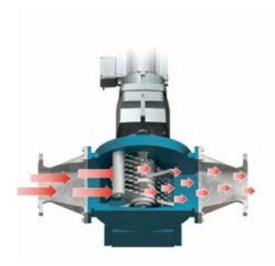
The Rotorrake tackles macerating tasks where others have failed – for macerating very coarse solids and rags. Coarse objects which cannot be macerated are ejected into the foreign body separator.
