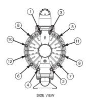
Inlet Manifold Torque bolts to 22–25 N•m
