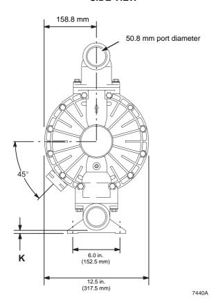
Dimensions B, C, F, G, H and M can vary by up to 1/4 in. (6.3 mm) depending on the seat and diaphragm material fitted in the pump.
