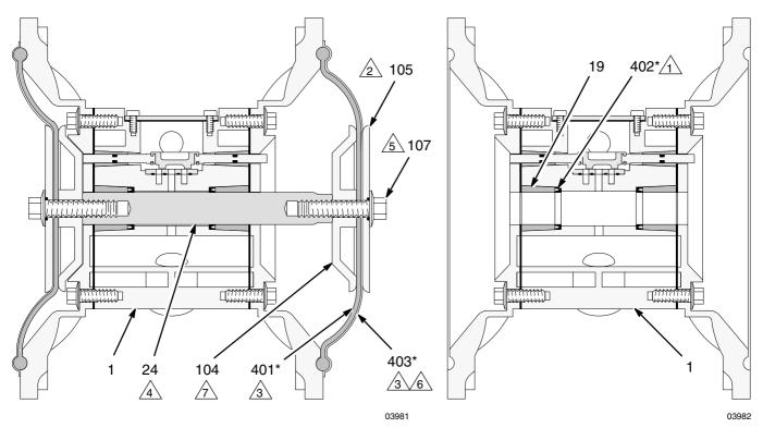
Cutaway View, with Diaphragms in Place
