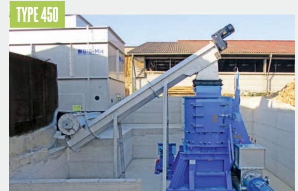
A two-part TYPE 450 screw conveyor system consisting of a horizontal and an inclined screw conveyor feeds a vertical shredder. The feed rate is individually adapted to the performance level of the downstream vertical shredder and the desired degree of shredding.
