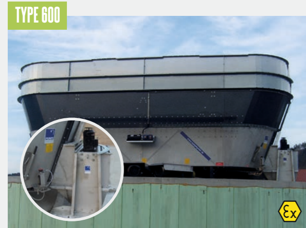
The fermenter screw TYPE 600 with vertical entry according to ATEX feeds the fermenter directly. The solids feeder transfers the substrate into the fermenter screw via a hydraulic slide opening
