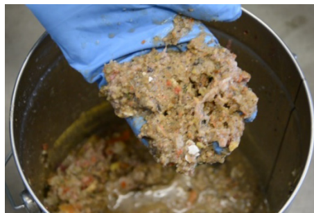
Kitchen waste after it has been macerated → Result makes discharge into the sea possible
