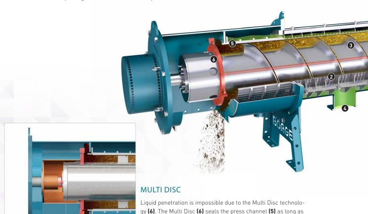
the required drying stage of the thick matter plug is achieved. This is when the slot for discharging opens and the solid phase is loosened and expelled – **penetration-proof technology.**
