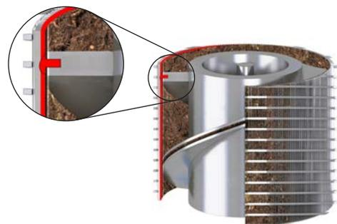
Fibers are caught in the patented profile groove of the auger, where they function as a brush. Metallic rubbing between the auger and the wedge wire screen is avoided by this brush.
