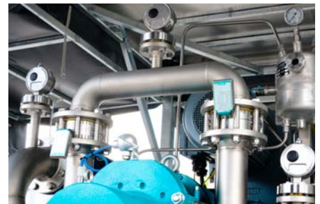
Overpressure protection by bypass with rupture disks
